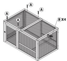
Attach top panel using screw A. Attach lock using screw B.
