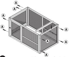
Use screw A to connect the front and back panels to the side panels. Drop in roosting bar.
