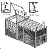
Attach large roof with screw E. Attach small roof with with screw D. Attach hinges to coop roof with provided screws.
