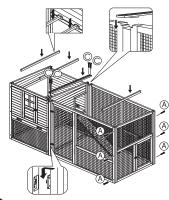
Attach front and back wire panels to side wire panel with screw A. Lock wire panels to connector bars as shown. Attach top connector bar with screw C. Add roosting bars.
