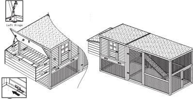
Slide in the nesting box lid as shown. Make sure the hinge joints connect properly. Attach the safety catch hinge with provided screws.
