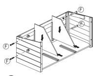
Use bolt F to assemble the nesting box. Insert floor panel in the direction shown. Use bolt G to connect the nesting box to the main house then insert the divider panel.
